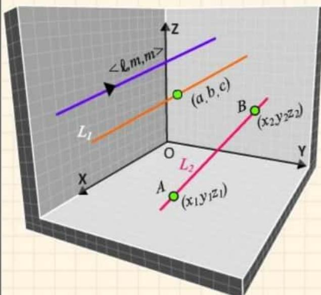
Line passing through point  $(a, b, c)$  parallel to line having direction cosines  $\ell, m, n$  is
